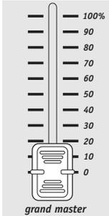
Pilot 2000 has a general output level control, by means of which the overall level of all the “dimmer” channels is regulated (both of the conventional type and those of intelligent units). The value is expressed as a percentage, ranging from 0 to 100%
