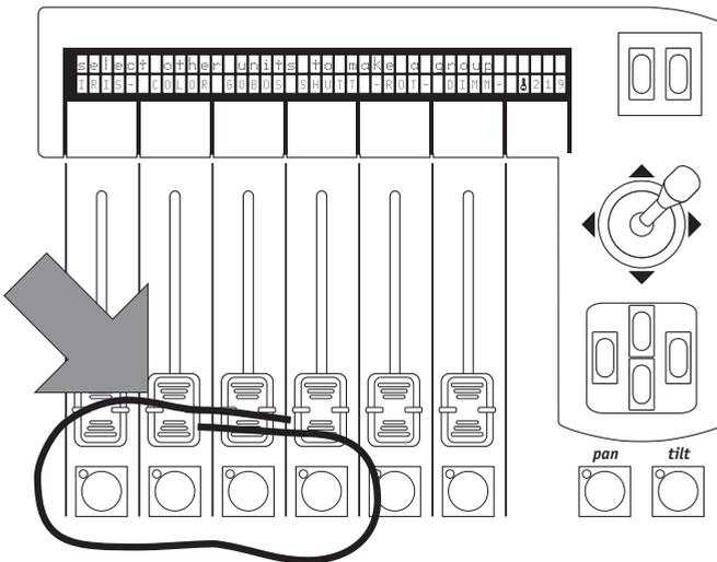
6 - Set the levels required per each channel using the universal faders.
